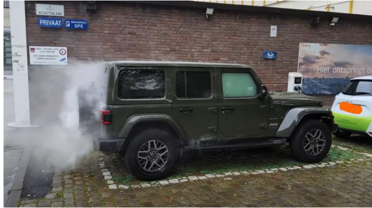
Figure 26 Example of a vehicle that has filled with battery vent gases – note the white smoke.
