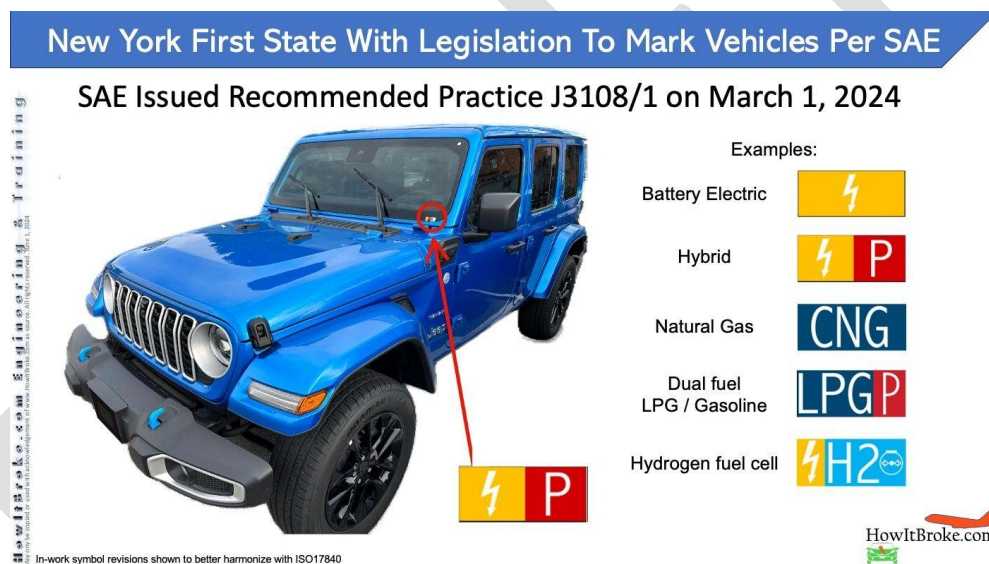
Figure 13 Slide showing an example of the SAE J3108 window sticker location and selected examples (courtesy of Bob Swaim). 58
