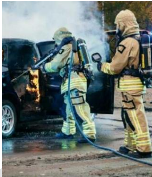
Figure 24 Photograph showing the application of the water lance with extension on an EV fire.
