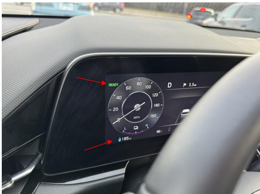
Figure 19 Instrument panel of a Kia Niro, as viewed from the driver's side doorway. Note the green "READY" indicating that the HV battery can supply power to the inverter/wheels, air conditioning, or other HV consumers.
