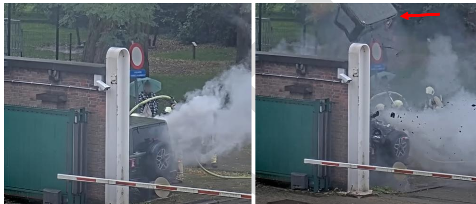
Figure 16 Screenshot of a video showing white fog emanating from a vehicle (left), followed by a screenshot after an explosion occurred where the roof of the cab has been pushed off of the vehicle (see red arrow). First-responders opened a window or door prior to the incident to ventilate the cabin. 72
